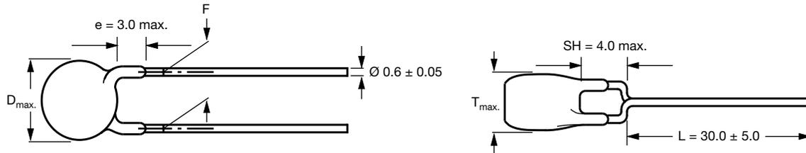
Capacitors with 10.0 mm or 12.5 mm lead spacing
