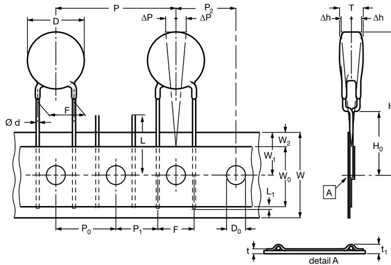
The sprocket hole pitch ( $P_0$ ) is 12.7 mm for lead spacing 10.0 mm and 12.5 mm
