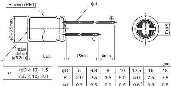
\*In case L > 25 for the φ12.5 dia. unit, lead dia.  $\phi d = 0.8$ mm.
