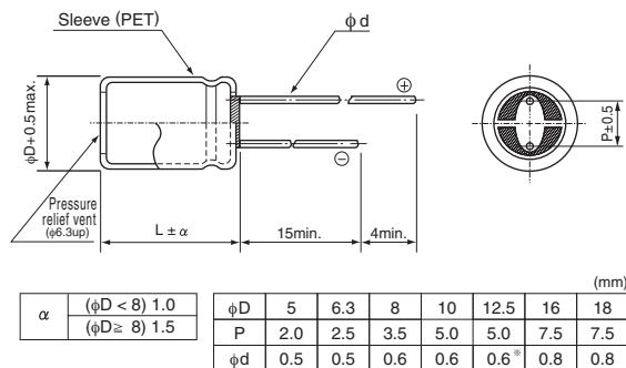
※ In case L > 25 for the φ12.5 dia. unit, lead dia. φ d=0.8mm.
