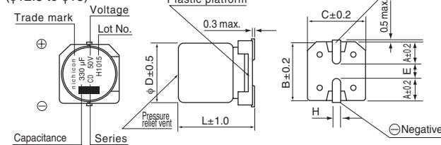
For φ8×10L, φ10×10L, φ12.5×13.5L, φ16×16.5L, and φ18×16.5L, some part numbers can be produced vibration-resistant construction. Please contact us for details.
