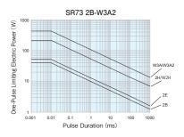
The maximum applicable voltage is equal to the max. overload voltage. Please ask us about the resistance characteristic of continuous applied pulse. The pulse endurance values are not assured values, so be sure to check the products on actual equipment when you use them.
