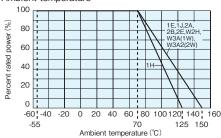
For resistors operated at an ambient temperature of  $70^{\circ}$ C or higher, the power shall be derated in accordance with the above derating curve.
