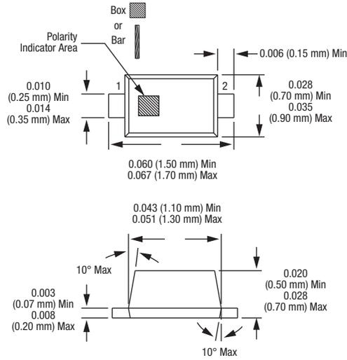
Dimensions are in inches (millimeters shown in parentheses) 200046-007
