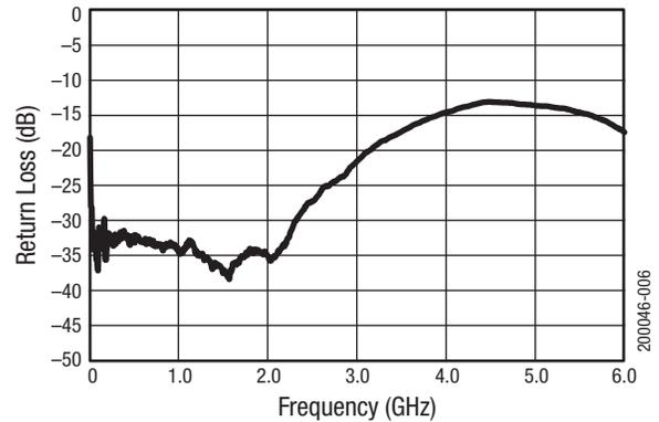
**Figure 6. Return Loss vs Frequency
