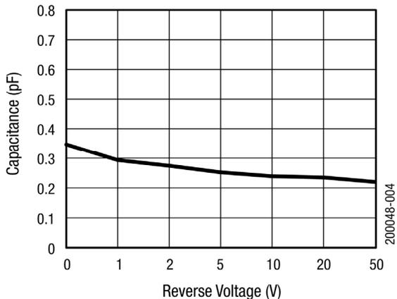
**Figure 3. Capacitance vs Reverse Voltage (1 MHz to 1 GHz)**
