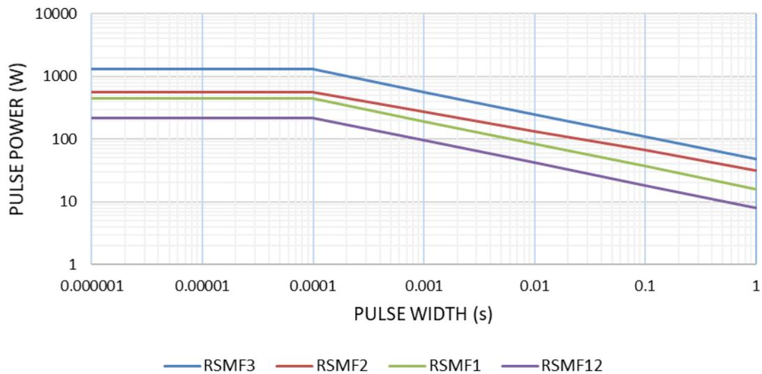
**Pulse Limiting Power (one pulse) / RSMF Series > 5Ω**
