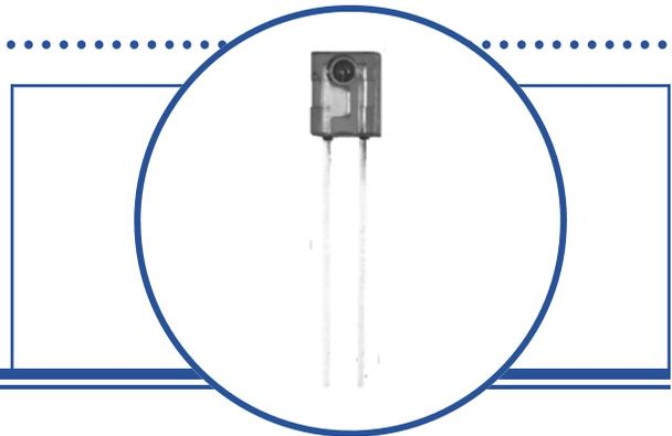
The OPV382 is a Vertical Cavity Surface Emitting Laser (VCSEL) packaged in a dome lens lateral package. VCSELs offer many advantages in sensing applications when compared to infrared LEDs. These devices require substantially lower drive currents to obtain the same amount of output power as LEDs. This feature allows VCSELs to be used in low power consumption applications such as battery operated equipment.
