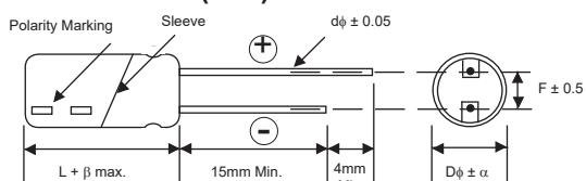
$$\beta = L < 20\text{mm} = 1.5\text{mm}, L \geq 20\text{mm} = 2.0\text{mm}$$
