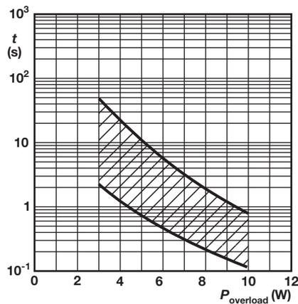
**NFR25** This graph is based on measured data which may deviate according to the application.
