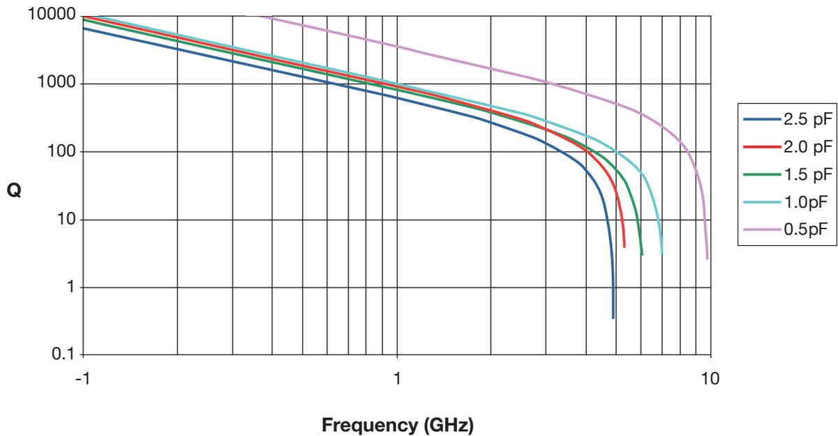
Typical Self Resonant Frequency vs. Capacitance
