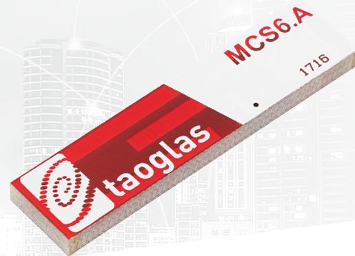
The MCS6.A is a low profile SMD NB-IoT / CAT M1 Bands / 4G/3G/2G embedded antenna designed for direct SMD mount on a device PCB. It provides high efficiency in a very small form factor of just 42\*10\*3mm.
