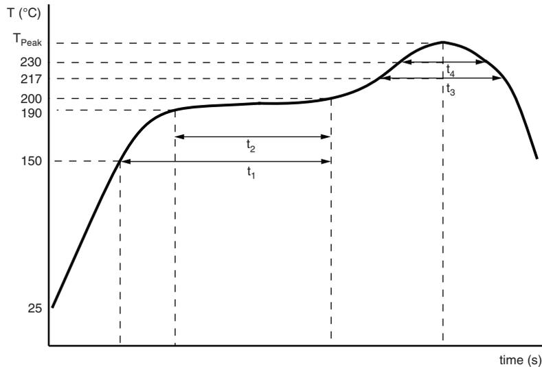
Fig. 4 - Maximum temperature load during reflow soldering
