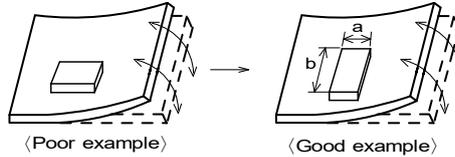
(2) Components location on PCB separation
