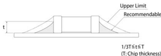
An increased solder volume increases mechanical stress on the product. Exceeding solder volume may cause the failure of mechanical or electrical performance.
