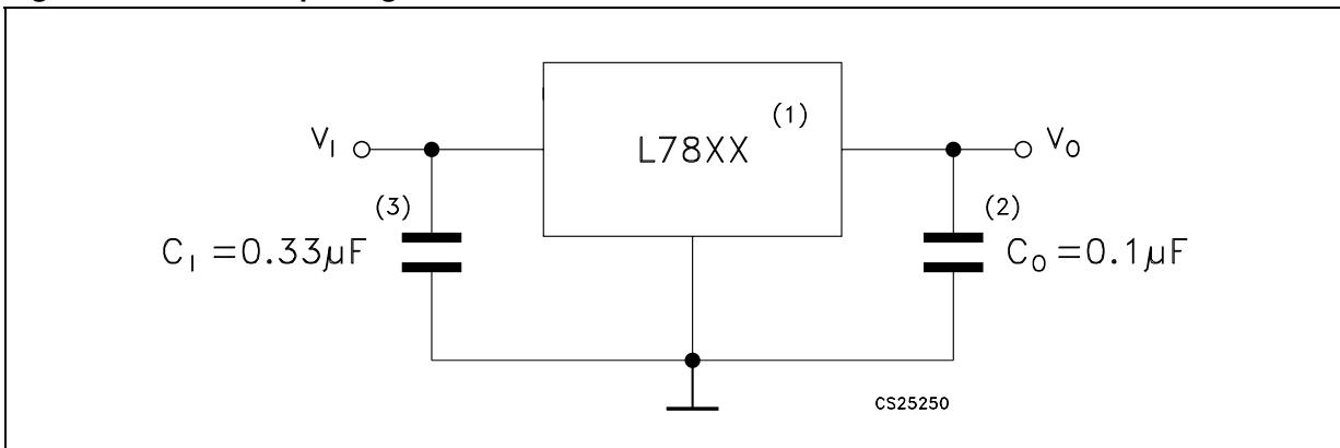
1. To specify an output voltage, substitute voltage value for "XX".
