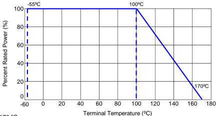
Operating temperature range of -55 to 170  $^{\circ}$ C. Storage condition: 5 ~ 35  $^{\circ}$ C, humidity of 40 ~ 75%.
