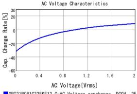
GRT21BC81C335KE13 C-AC Voltage capchange, DCOV, 25.0d
