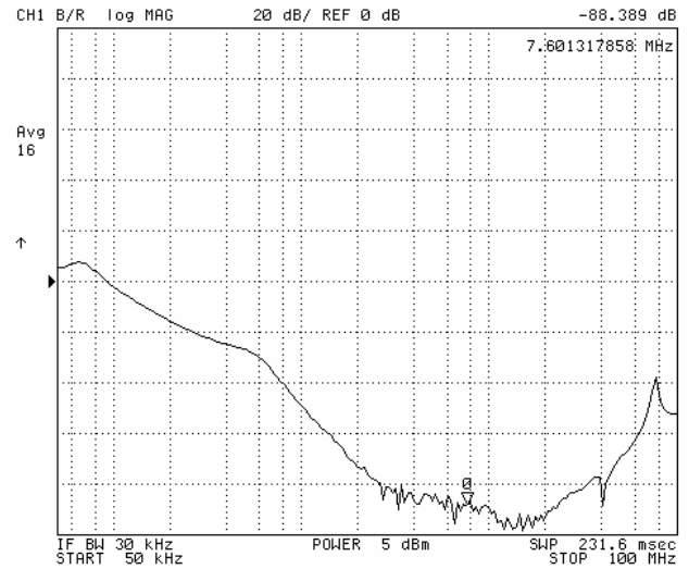
Fig. 3: Common Mode attenuation, 0.05-100 MHz. Source and load resistances are 50 \Omega . Two 0.1 \mu F Y-caps to common line. Vertical scale: 20 dB/div, with zero dB level marked by arrow.
