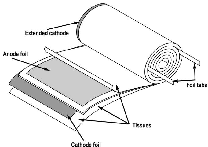
The deck, complete with terminals, is attached to the tabs and then folded down to rest on top of the winding. The complete winding is impregnated with electrolyte before being housed in a suitable container, usually an aluminum can, and sealed. Throughout the process, all materials inside the housing must be maintained at the highest purity and be compatible with the electrolyte.
