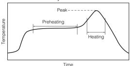
For soldering (Example: Sn/Pb)
