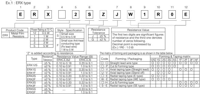
The above example 1 shows a small metal film resistor, 2 W power rating, resistance value of 1.0  $\Omega$ , tolerance  $\pm 5$  %, and package of radial taping
