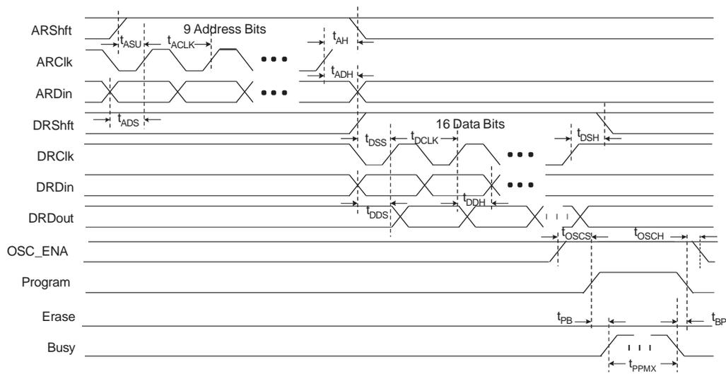
Figure 5-5. UFM Erase Waveform
