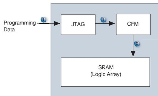
In real-time ISP mode, the user flash memory (UFM), programmable logic, and I/O pins remain operational while programming of the CFM is in progress. The contents of the CFM will not download into the SRAM after the successful programming of the CFM. Instead, the device waits for a power cycle to occur. The normal power-up sequence occurs (CFM downloads to SRAM at power-up) and the device enters user mode after  $t_{\text{CONFIG}}$  time. Figure 12-2 shows the flow of real-time ISP.
