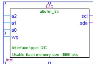
Figure 9-23 shows page 3 of the altufm MegaWizard Plug-In Manager when selecting I<sup>2</sup>C as the interface. On this page, you can choose whether to implement the read/write mode or read-only mode for the UFM. You also have an option to choose the memory size for the altufm\_i2c megafunction as well as defining the four MSBs of the slave address (default 1010).
