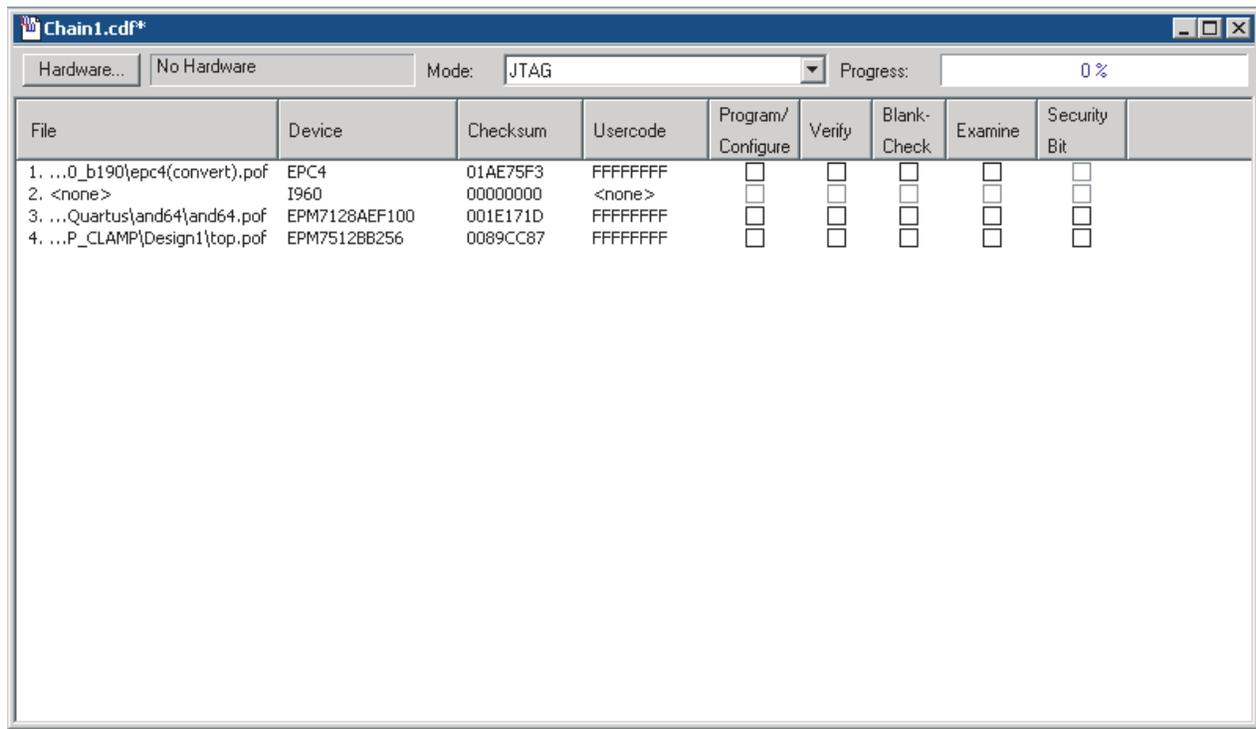
Figure 14-4. Generating a JBC File for a Multi-Device JTAG Chain in the Quartus II Software
