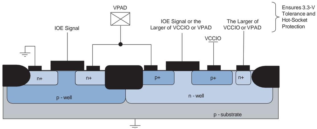
The CMOS output drivers in the I/O pins intrinsically provide electrostatic discharge (ESD) protection. There are two cases to consider for ESD voltage strikes: positive voltage zap and negative voltage zap.
