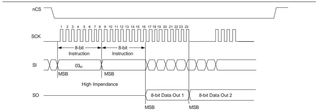
Figure 9-29 shows the WRITE operation sequence for Base mode.
