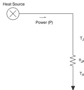
The PowerPlay Early Power Estimator spreadsheet determines the junction-to-ambient thermal resistance ( $\theta_{JA}$ ) based on the device, package, and airflow selected in the main input parameters.
