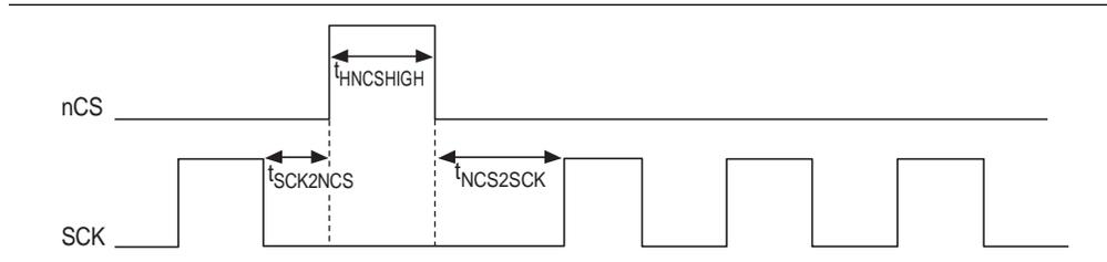
**Table 9-14.** SPI Timing Parameters for Extended Mode
