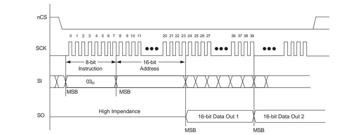
Figure 9-27 shows the READ operation sequence for Base mode.
