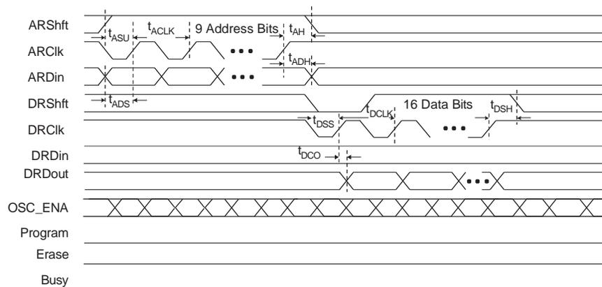
Figure 5-4. UFM Program Waveforms
