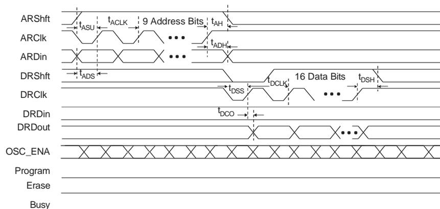
Figure 9-8. UFM Stream Read Waveforms
