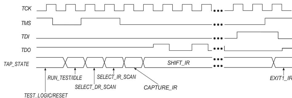
The TDO pin is tri-stated in all states except the SHIFT\_IR and SHIFT\_DR states. The TDO pin is activated at the first falling edge of TCK after entering either of the shift states and is tri-stated at the first falling edge of TCK after leaving either of the shift states.
