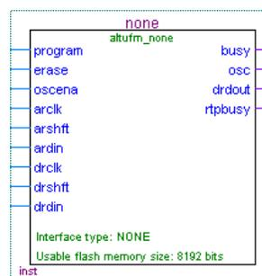
Figure 9-44 shows page 3 of the altufm MegaWizard Plug-In Manager, selecting **none** for the interface protocol. By selecting **none**, all the other options are grayed out or unavailable to you. However, you still can specify the initial content of the UFM block on page 4 of the altufm MegaWizard Plug-In Manager as discussed in “Creating Memory Content File” on page 9-40.
