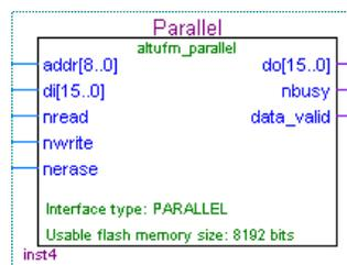
Figure 9-42 shows page 3 of the altufm MegaWizard Plug-In Manager, selecting the Parallel Interface as the interface. On this page, you can choose whether to implement the Read/Write mode or Read Only mode for the UFM. You also have an option to choose the width for address bus (up to 9 bits) and for the data bus (up to 16 bits). You can specify the initial content of the UFM block on page 4 of the altufm MegaWizard Plug-In Manager as discussed in “Creating Memory Content File” on page 9-40.
