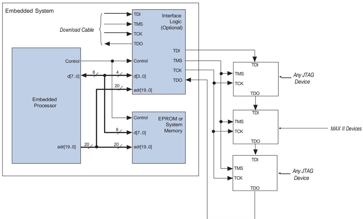
Both JTAG connection methods should include space for the MasterBlaster™, ByteBlaster™ II, or USB-Blaster™ header connection. The header is useful during prototyping because it allows designers to quickly verify or modify the PLD's contents. During production, the header can be removed to decrease cost.
