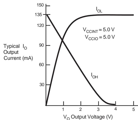
As shown above,  $R_1 = 5.0 \text{ V}/135 \text{ mA}$ .
