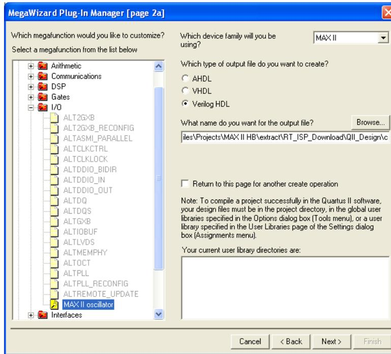
Figure 9-6 shows page 3 of the IO/MAX II oscillator megafunction. You have an option to choose to simulate the OSC output port at its maximum or minimum frequency during the design simulation. The frequency chosen is only used as a timing parameter simulation and does not affect the real MAX II device OSC output frequency.
