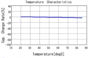
DE21XSA220KN3AX02F C-Temp. capchange, DC0V, AC1Vrms
