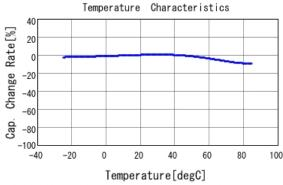
DE1B3RA221KN4AQ01F C-Temp. capchange, DC0V, AC1Vrms
