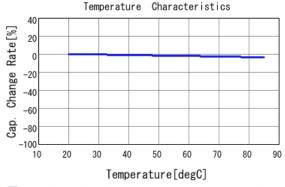
DE11XRA470KN4AN01F C-Temp. capchange, DC0V, AC1Vrms
