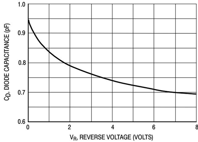
Figure 3. Diode Capacitance
