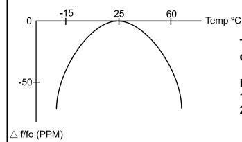
To calculate the frequency stability the parabolic curvature constant (K) is needed.
