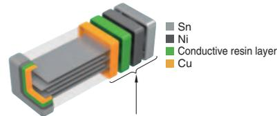
The conductive resin layer covers overall surface of copper.
