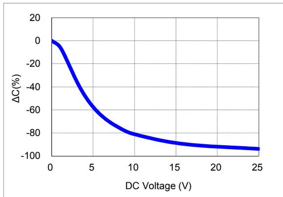
4) Bias TCC characteristics (Agilent 4284A, 1kHz, 0.5Vrms, 12.5Vdc)
