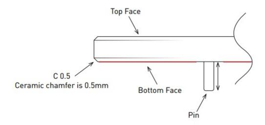
Red Line shows the adhesive without Liner - thickness 0.08~0.1mm
