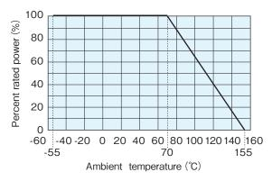
For resistors operated at an ambient temperature of  $70^{\circ}\text{C}$  or higher, the power shall be derated in accordance with the above derating curve.
