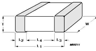
Fig. 2 Surface mounted multilayer ceramic c
