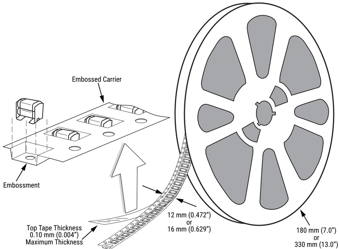
**Table 5 – Carrier Tape Configuration – Embossed Plastic (mm)**
