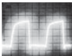
Signal Waveform (20ns/div, 1V/div)
