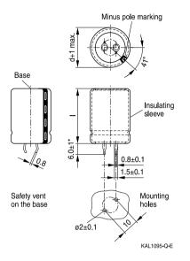
Snap-in terminals, length (6.0  $\pm$ 1) mm. Also available in a shorter version with a length of (4.5 -1) mm.
