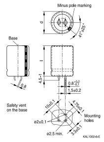
Snap-in capacitors are also available with 3 terminals (length (4.5 - 1) mm).
