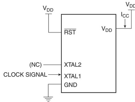
26.13.5 Clock Signal Waveform for  $I_{CC}$  Tests
