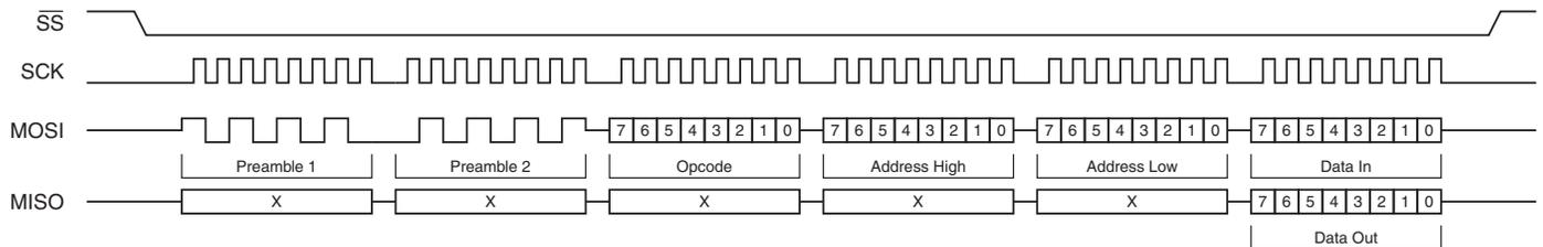
**Figure 25-6.** ISP Command Packet (Parallel)
