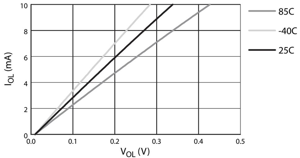
Note: The  $I_{OL}/V_{OL}$  characteristic applies to Push-Pull, Quasi-Bidirectional and Open-Drain modes.
