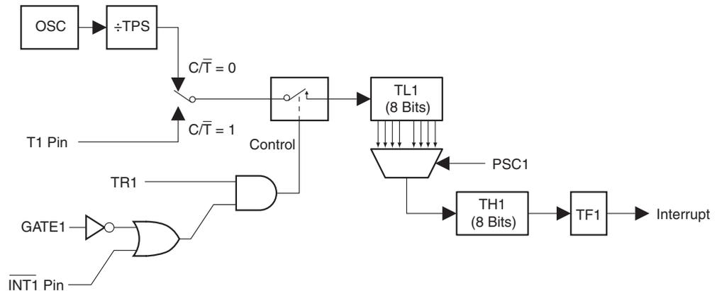
Mode 0 operation is the same for Timer 0 as for Timer 1, except that TR0, TF0, GATE0 and  $\overline{\text{INT0}}$  replace the corresponding Timer 1 signals in [Figure 11-1](#). There are two different C/T bits, one for Timer 1 (TMOD.6) and one for Timer 0 (TMOD.2).
