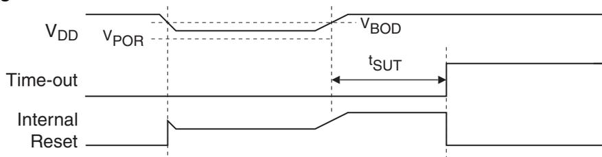
The AT89LP3240/6440 allows for a wide  $V_{\text{DD}}$  operating range. The on-chip BOD may not be sufficient to prevent incorrect execution if  $V_{\text{BOD}}$  is lower than the minimum required  $V_{\text{DD}}$  range, such as when a 3.6V supply is coupled with high frequency operation. In such cases an external Brown-out Reset circuit connected to the  $\overline{\text{RST}}$  pin may be required.
