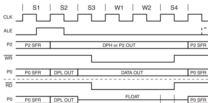
**Figure 3-13. MOVX with Three Wait States (WS = 11B)**
