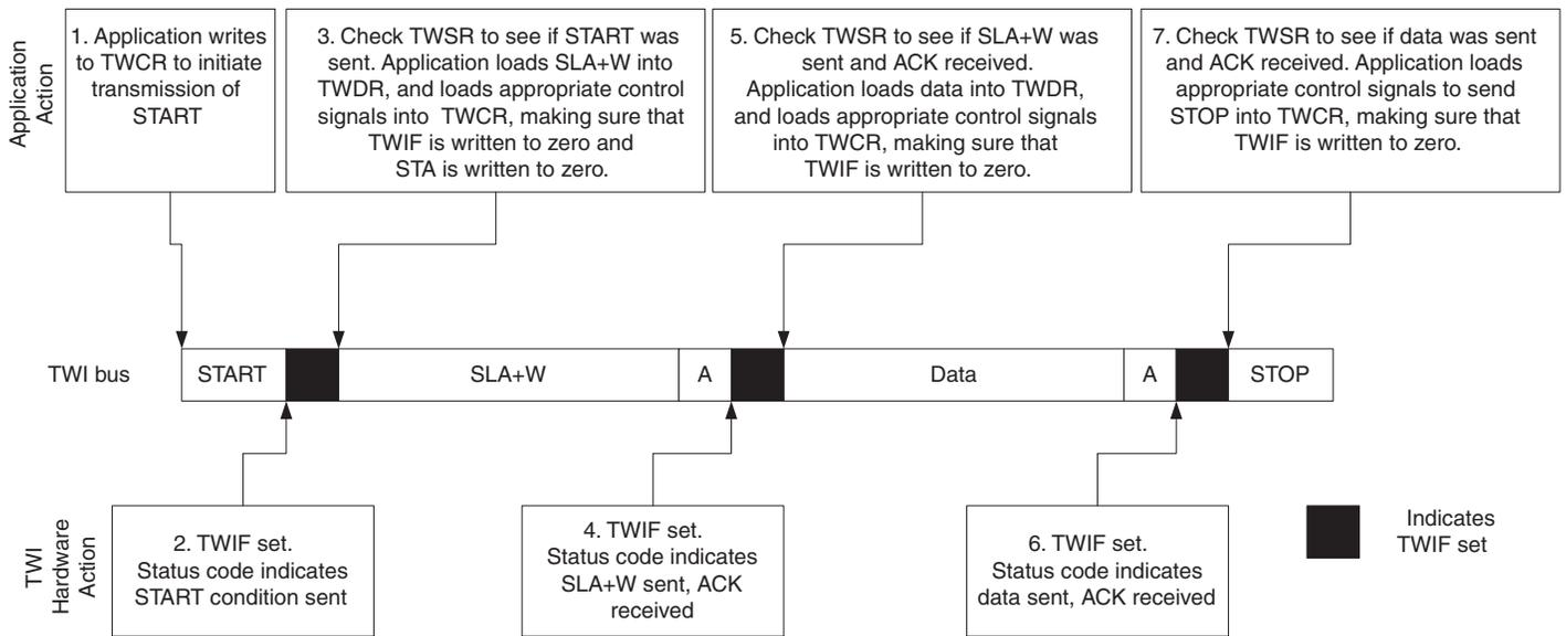
1. The first step in a TWI transmission is to transmit a START condition. This is done by writing a specific value into TWCR, instructing the TWI hardware to transmit a START condition. Which value to write is described later on. However, it is important that the TWIF bit is cleared in the value written. The TWI will not start any operation as long as the TWIF bit in TWCR is set. Immediately after the application has cleared TWIF, the TWI will initiate transmission of the START condition.
