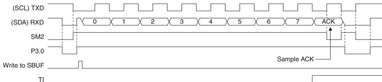
Mode 0 transfers data LSB first whereas SPI or TWI are generally MSB first. Emulation of these interfaces may require bit reversal of the transferred data bytes. The following code example reverses the bits in the accumulator:
