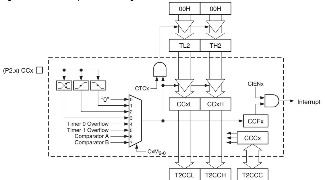
Each CCA channel has an associated external capture input pin: CCA (P2.0), CCB (P2.1), CCC (P2.2) and CCD (P2.3). External capture events are always edge-triggered and can be selected
