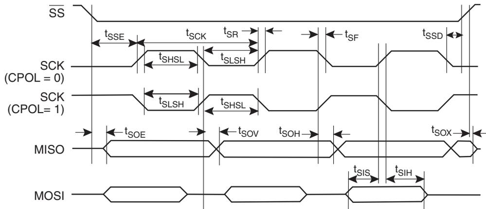
Figure 26-19. SPI Master Timing (CPHA = 1)
