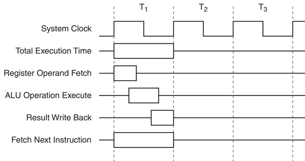
**Figure 5-3.** Two-cycle ALU Operation (Example: ADD A, #data)
