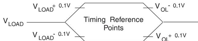
Note: 1. For timing purposes, a port pin is no longer floating when a 100 mV change from load voltage occurs. A port pin begins to float when 100 mV change from the loaded  $V_{OH}/V_{OL}$  level occurs.
