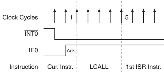
**Figure 9-2.** Maximum Interrupt Response Time
