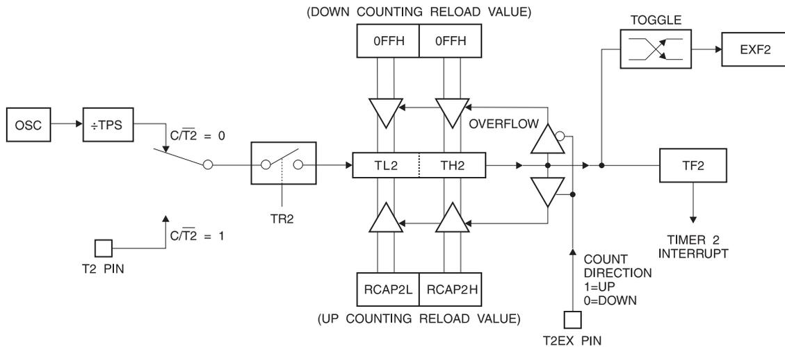
The timer overflow/underflow rate for up-down counting mode is the same as for up counting mode, provided that the count direction does not change. Changes to the count direction may result in longer or shorter periods between time-outs.
