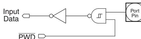
Figure 10-3. Input Circuit for P3.2, P3.3, P4.0, P4.1 and P4.2
