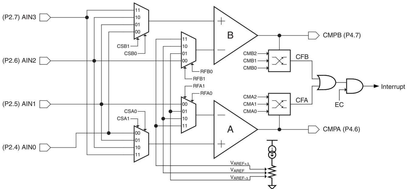
A block diagram of the dual analog comparators with relevant connections is shown in [Figure 19-1](#). Input options allow the comparators to function in a number of different configurations as shown in [Figure 19-4](#). Comparator operation is such that the output is a logic “1” when the positive input is greater than the negative input. Otherwise the output is a zero. Setting the CENA (ACSR.A.3) and CENB (ACSR.B.3) bits enable Comparator A and B respectively. The user must
