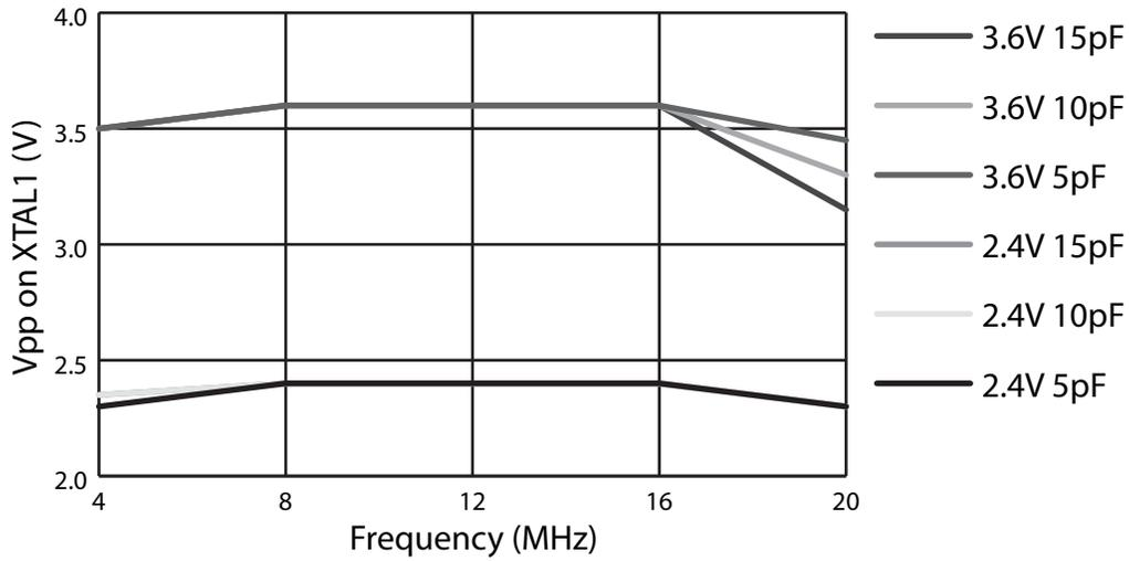
Note: 1. Replacing capacitor C1 with a resistor R1 of 4 MΩ results in similar swing levels on XTAL1.
