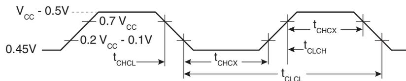
26.13.6  $I_{CC}$  Test Condition: Power-down Mode
