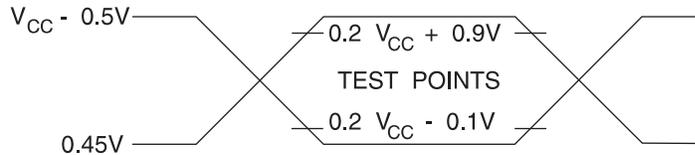
Note: 1. AC Inputs during testing are driven at  $V_{DD} - 0.5V$  for a logic "1" and  $0.45V$  for a logic "0". Timing measurements are made at  $V_{IH}$  min. for a logic "1" and  $V_{IL}$  max. for a logic "0".
