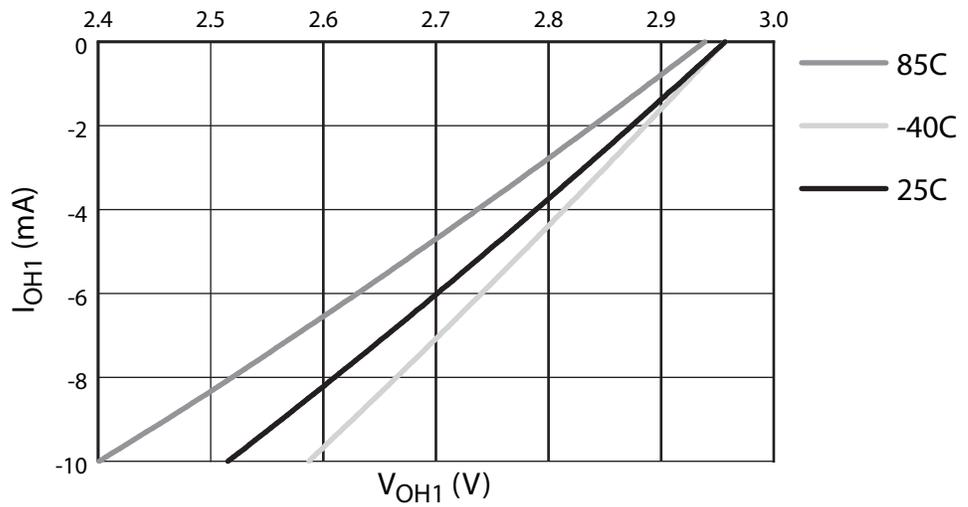
Figure 26-10. Push-Pull Output I-V Sink Characteristic at 3V
