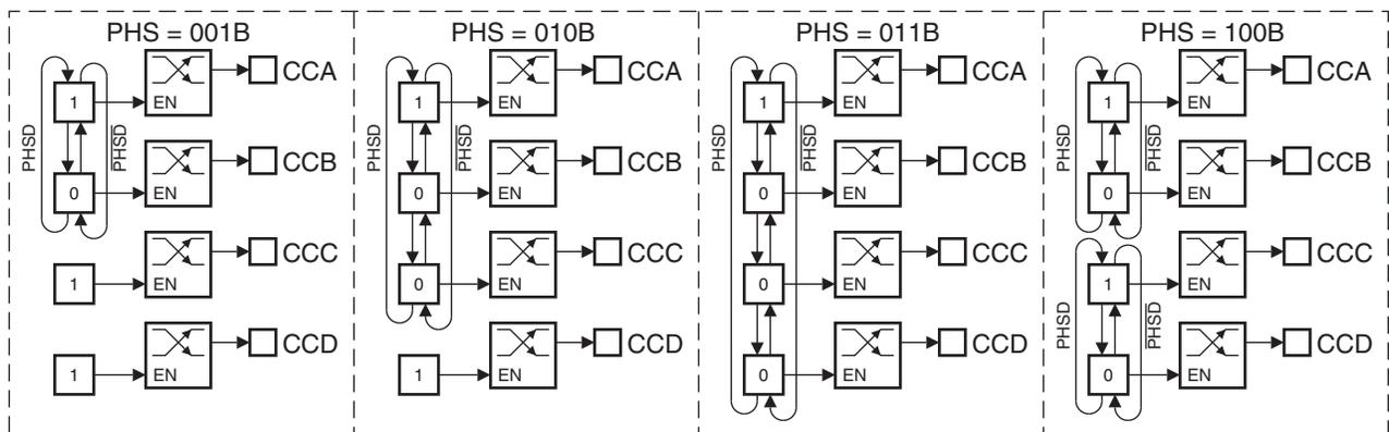
**Figure 13-13.** Three-Phase Mode with Channel B Disabled
