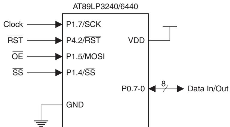
The Programming Interface is the only means of externally programming the AT89LP3240/6440 microcontroller. The Interface can be used to program the device both in-system and in a stand-alone serial programmer. The Interface does not require any clock other than SCK and is not limited by the system clock frequency. During Programming the system clock source of the target device can operate normally.
