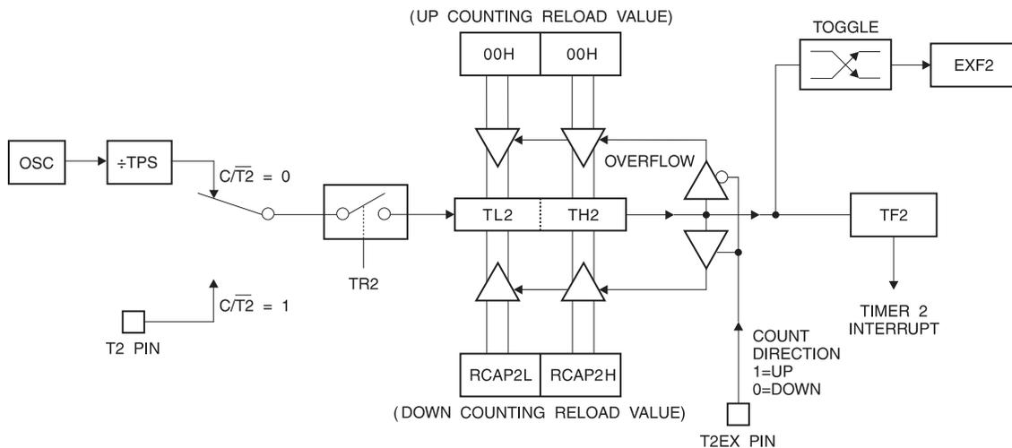
**Figure 12-6.** Timer 2 Waveform: Auto-Reload Mode (DCEN = 1)
