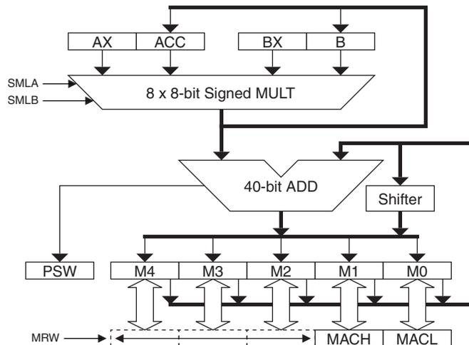
The MAC operation is performed by executing the MAC AB (A5 A4H) extended instruction. This two-byte instruction requires nine clock cycles to complete. The operand registers are not modified by the instruction and the result is stored in the 40-bit M register. MAC AB also updates the C and OV flags in PSW. C represents the sign of the MAC result and OV is the two's complement overflow. Note that MAC AB will not clear OV if it was previously set to one.
