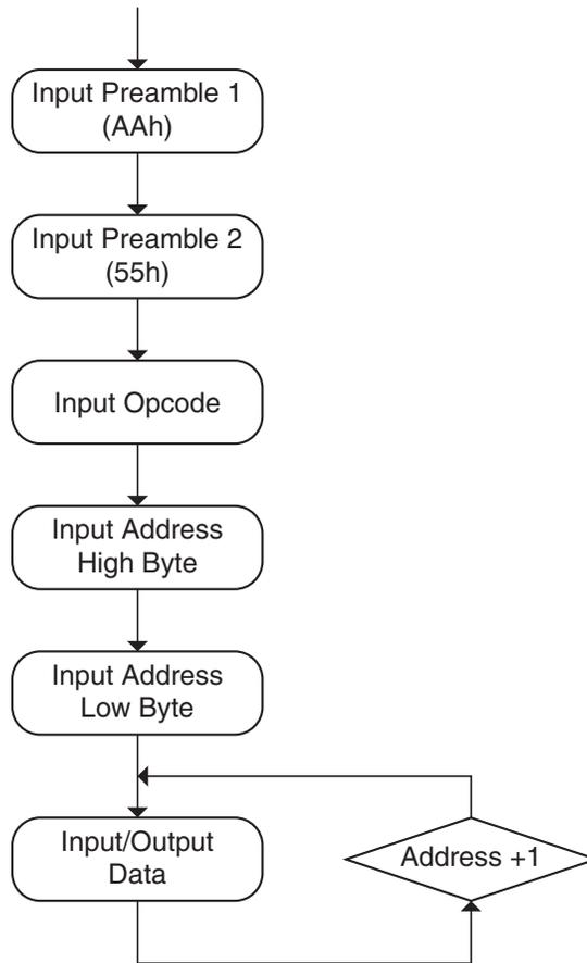
**Figure 25-5.** ISP Command Packet (Serial)
