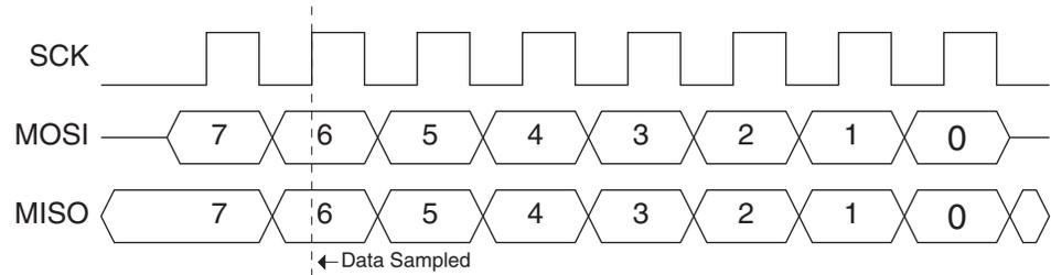
**Figure 25-12. Serial Programming Interface Timing**
