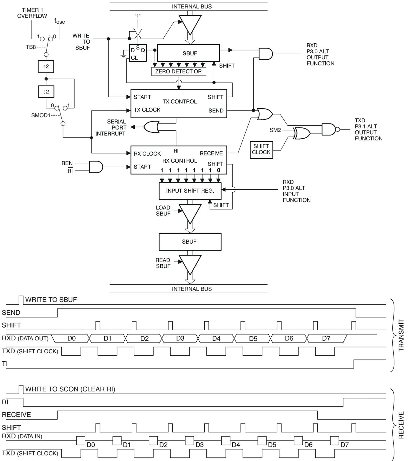
**Figure 16-2. Mode 0 Waveforms**
