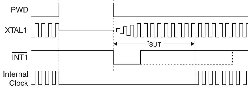
When PWDEX = “1”, the wake-up period is controlled externally by the interrupt. Again, at the falling edge on the interrupt pin, power-down is exited and the oscillator is restarted. However, the internal clock will not propagate until the rising edge of the interrupt pin as shown in [Figure 8-2](#). The interrupt pin should be held low long enough for the selected clock source to stabilize. After the rising edge on the pin the interrupt service routine will be executed.
