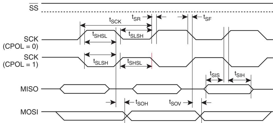
Figure 26-18. SPI Slave Timing (CPHA = 0)
