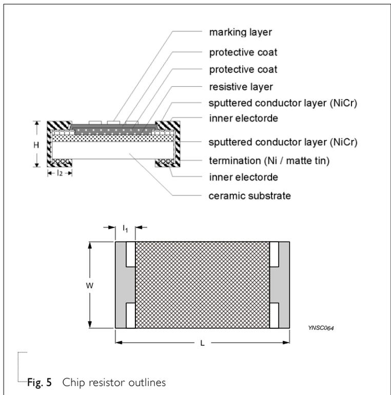
**Fig. 5** Chip resistor outlines
