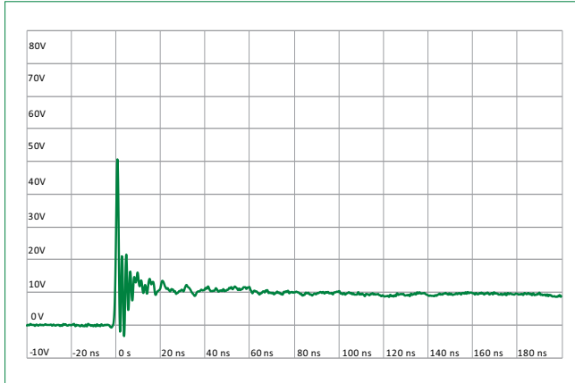
ISO10605 Contact Discharge Plot at +8 kV
