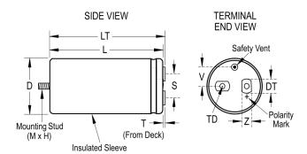
General Information Series ALS61 Dielectric Aluminum Electrolytic High Voltage, Screw Terminal, Aluminum Description Electrolytic Features High Voltage RoHS Yes Mounting Stud AEC-Q200 No **Typical Component** 505 g Weight Dimensions D And L Include Sleeving. MS Notes (MxH) = M12x16.
