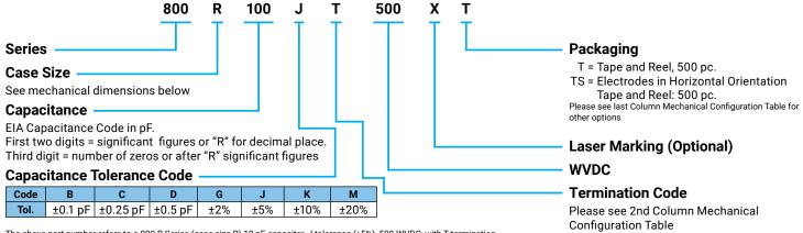
The above part number refers to a 800 R Series (case size R) 10 pF capacitor, J tolerance ( $\pm$ 5%), 500 WVDC, with T termination (Tin Plated over Nickel Barrier, RoHS Compliant), laser marked, and tape and reel packaging.
