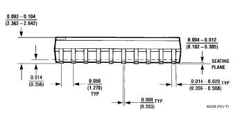
Figure 2. 20-Lead Small Outline Integrated Circuit (SOIC), JEDEC MS-013, 0.300" Wide Package Number M20B
