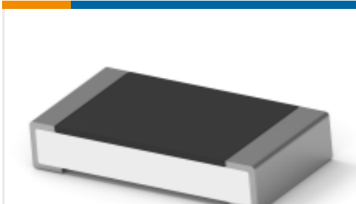
TE Part # 1-2176391-0 RQ 1206 15K4 0.1% 10PPM 5K RL
