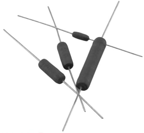
Ohmite 40 Series resistors are the most economical conformal silicone-ceramic coated resistors offered. These all-welded units are characterized by their low temperature coefficients and resistance to thermal shock, making them ideal for a wide range of electrical and electronic applications.
