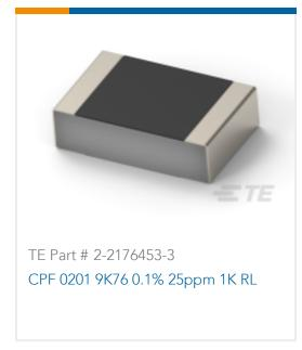
Precision Resistor, Thin Film, 0201, .0313 W, 100  $\Omega$ , .1 %, ±25 ppm/°C, Solder, 2 Termination, Height .009 in [.23 mm], Neohm CPF
