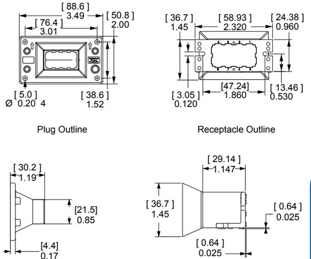
See APP's innovative MARC Connector that offers straight-on or rotational blindmate capability. MARC holds 6 PP15/45 power contacts and 2 PP15/45 premate ground contacts in a high temperature housing. Visit our website, [www.andersonpower.com](http://www.andersonpower.com) to learn more.
