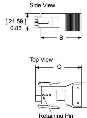
**NEW Plug Shell with Latch & Non-Conductive Strain Relief**
