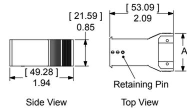
NOTE: Retaining pins are used to secure and position Powerpoles® in one of three positions in plug shells.
